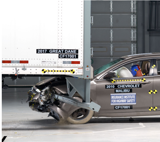
Great Dane made improvements to its rear underride guard to successfully prevent underride in the IIHS 30 percent overlap test.
