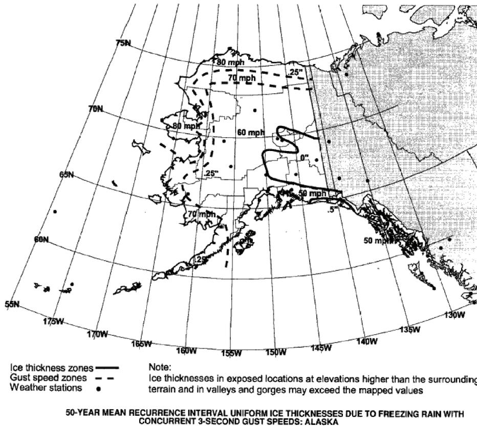
**Figure 250-3(f)—Uniform ice thickness with concurrent wind**
