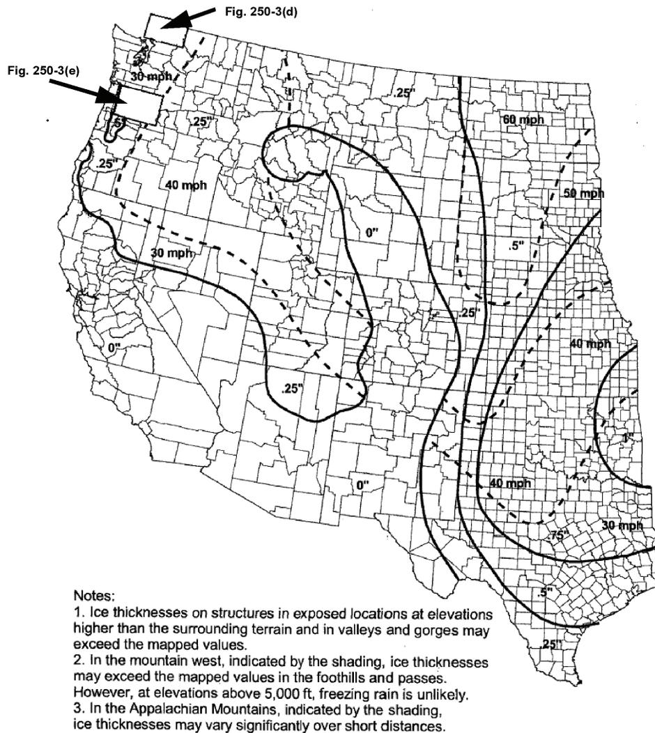
**50-YEAR MEAN RECURRENCE INTERVAL UNIFORM ICE THICKNESSES DUE TO FREEZING RAIN WITH CONCURRENT 3-SECOND GUST SPEEDS: CONTIGUOUS 48 STATES.**
