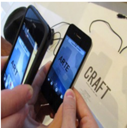
Using the Word Lens app to translate the word "Craft" in real-time. (Image source: http://www.flickr.com/photos/neven/5269418871/ )
