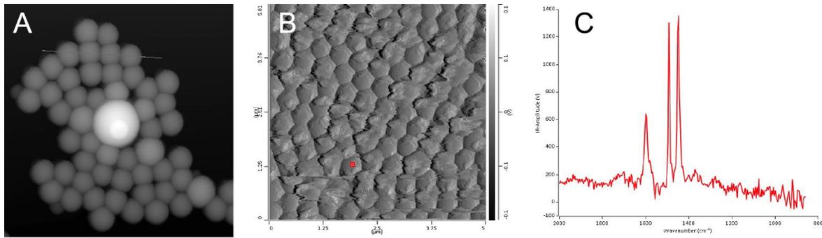
**Figure 7.** (A) A monolayer of beads visualized using AFM. (B) Red dot indicates polystyrene bead from which spectrum generated in panel C was obtained. (C) IR spectrum indicating characteristic peaks of polystyrene at  $1452\text{ cm}^{-1}$  and  $1492\text{ cm}^{-1}$ . Data generated by Rachel Merzel, Banaszak Holl Lab (University of Michigan).
