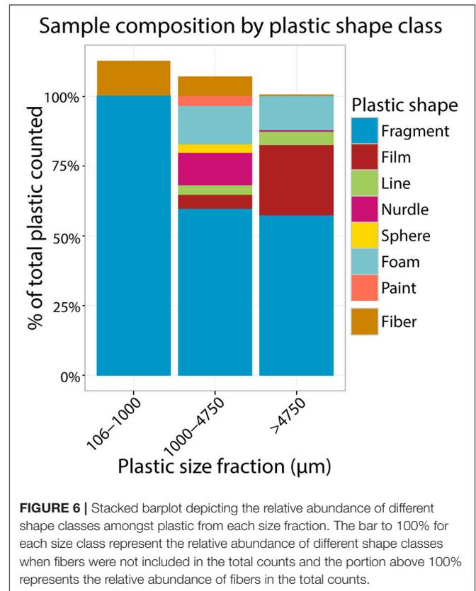
**FIGURE 6** | Stacked barplot depicting the relative abundance of different shape classes amongst plastic from each size fraction. The bar to 100% for each size class represent the relative abundance of different shape classes when fibers were not included in the total counts and the portion above 100% represents the relative abundance of fibers in the total counts.
