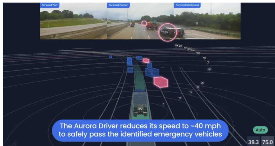
An Aurora autonomous truck safely and accurately detects an emergency vehicle, slows down, and changes lanes. 24
