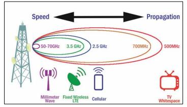
Figure 3: Simple Propagation Diagram
